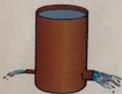
Figure 34.4 ▲ For a given pressure, more water passes through a large pipe than a small one. Similarly, for a given voltage, more electric current passes through a large-diameter wire than a small-diameter one.
