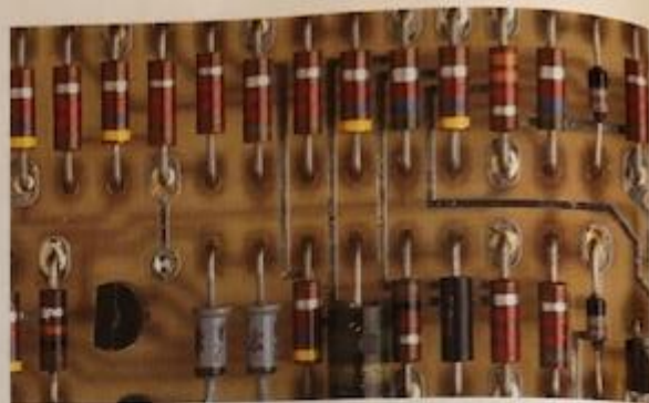
Figure 34.6 ▲ Resistors. The stripes are color coded to indicate the resistance in ohms.
