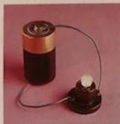
Figure 34.3 ▲ Each coulomb of charge that is made to flow in a circuit that connects the ends of this 1.5-volt flashlight cell is energized with 1.5 joules.
